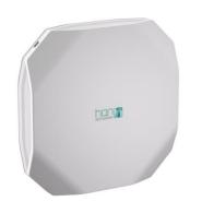
AP321 supports a maximum concurrent data rate of 2.975Gbps (2.402Gbps in 5GHz and 573Mbps in 2.4GHz), six spatial streams (2SS in 2.4GHz and 4SS in 5GHz), 160(80+80)MHz channels, and all Wi-Fi 6 (802.11ax) features, UL/DL MU-MIMO, UL/DL OFDMA, BSS color, etc. Enables faster speeds, more capacity, and efficient airtime allocation for clients on both 2.4Ghz and 5Ghz Wi-Fi bands.
