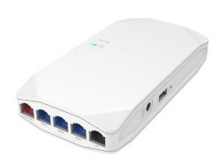
AP311H supports a maximum concurrent data rate of 1.775Gbps (1.201Gbps in 5GHz, and 574Mbps in 2.4GHz), four spatial streams (2SS in 2.4GHz and 2SS in 5GHz), and all Wi-Fi 6 (802.11ax) features, MU-MIMO, OFDMA, BSS color, etc. Enables faster speeds, more capacity, and efficient airtime allocation for clients on both 2.4Ghz and 5Ghz Wi-Fi bands.
